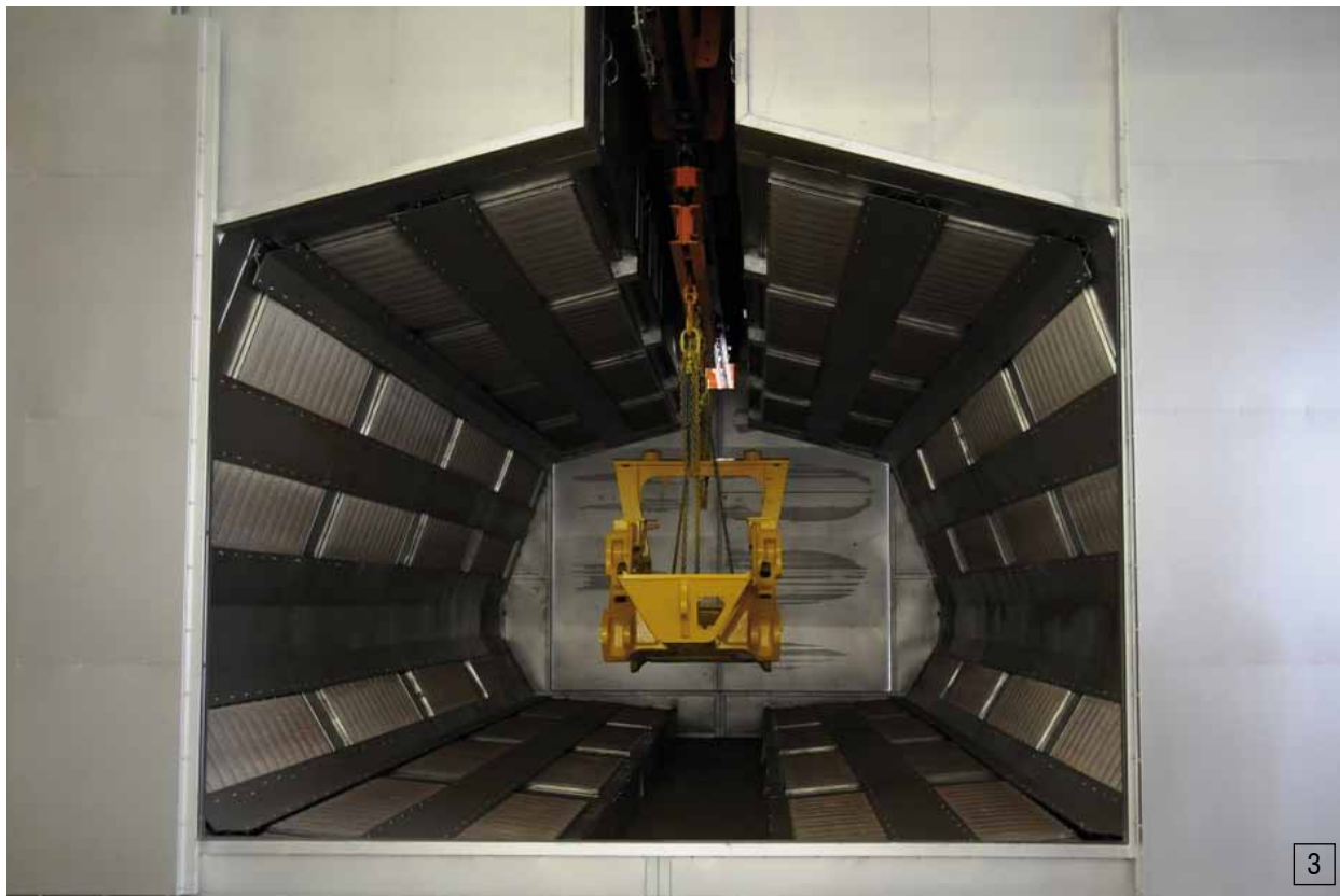
3 - Drying of liquid coating on "chassis" for earth moving machines
